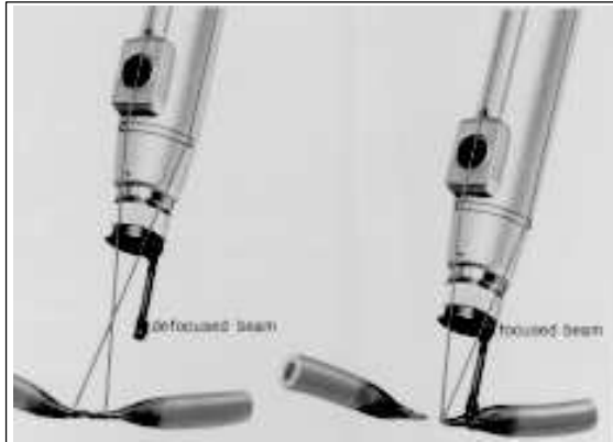
Larger defocused spots are associated with lower power densities and “cooking” or shrinkage of tissues. Smaller focused spots are associated with higher power densities and cutting of tissues
