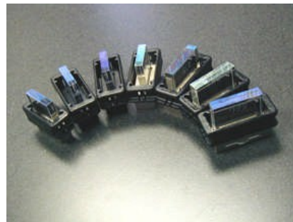
Various filters used to select certain wavelength bands
