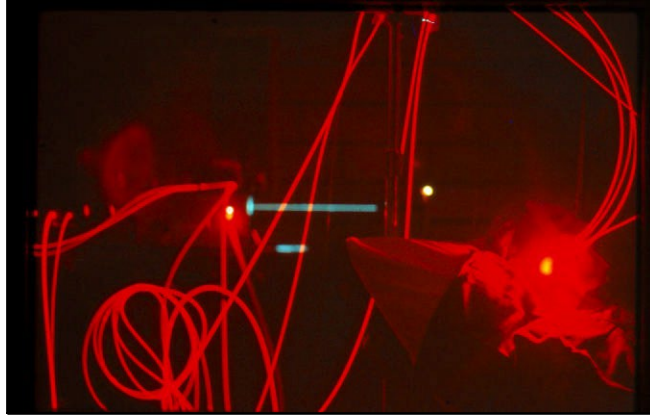
Argon Pumped Dye Laser for Photodynamic Therapy of Cancer Courtesy of Jim McCaughan, MD
